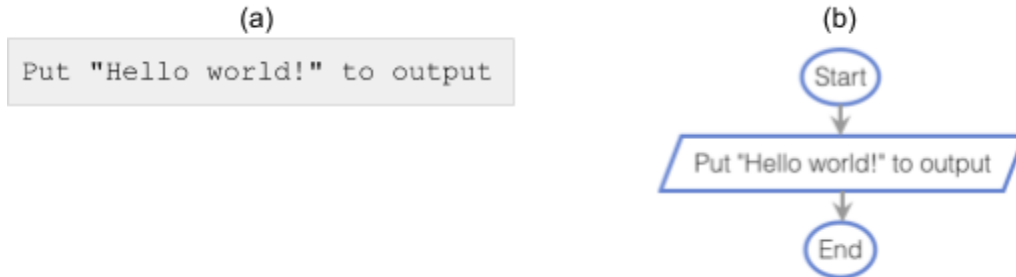
Figure 1: Example of string literal output in Coral for (a) textual code and (b) flowchart.
