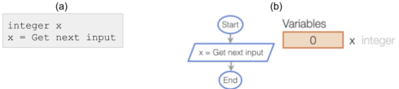
Figure 3: Example of getting the next input as (a) textual code and (b) flowchart.
